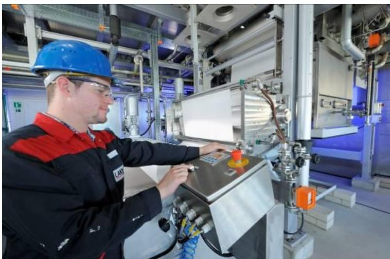
LANXESS is producing Lewabrane membrane elements for water treatment in Bitterfeld, Germany. The membrane's active separating layer forms a wafer-thin polyamide film. That filters out undesirable substances from water such as salts, pesticides, herbicides, viruses, bacteria and also minute particles. Photo: LANXESS AG
