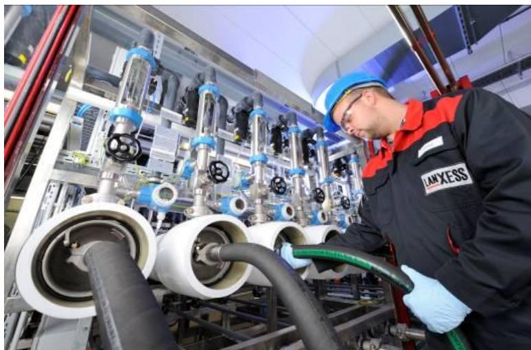
For quality assurance purposes each individual Lewabrane product is checked in an element tester at the LANXESS site in Bitterfeld, Germany. Photo: LANXESS AG
