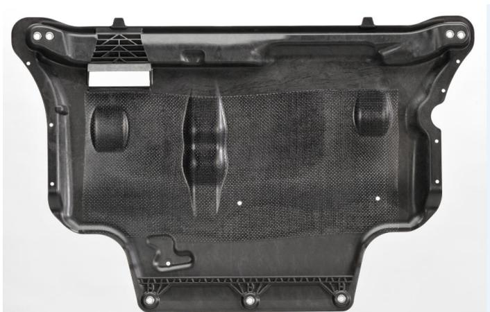
The engine undertray is made of a particularly robust thermoplastic composite design. This consists of the continuous-fiber-reinforced thermoplastic composite Tepex dynalite from specialty chemicals company LANXESS combined with a DLFT mass.
