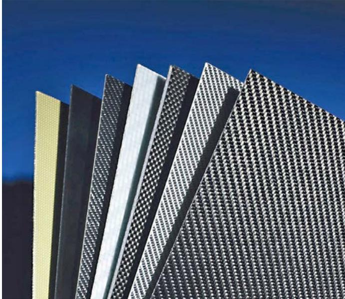
Semi-finished products of the continuous fiber-reinforced thermoplastic composites of the Tepex brand from LANXESS are ideal for structural lightweight design. As Tepex dynalite 102-RG600 they were also employed in the award-winning BMBF project FuPro.
