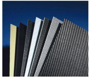
Tepex-brand continuous-fiber-reinforced composites are ideal for lightweight construction. Key markets include the automotive and electronics industries. They are also used in the sports and leisure sector. Photo: LANXESS AG
