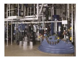
The cGMP plant O10 of Saltigo GmbH in Leverkusen for manufacturing active pharmaceutical ingredients (APIs) and intermediates obtained GMP (Good Manufacturing Practice) recertification in September 2017 with "no findings". The picture shows an eight-cubic-meter glass-lined vessel at the reactor level in the ultramodern multipurpose plant. Photo: Saltigo GmbH
