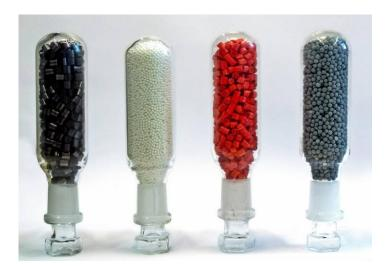
Standard forms of appearances of heterogeneous catalysts (from left to right): metal oxide catalyst in pelletized form, spherical, oxidic support, extruded catalyst support and support impregnated with precious metal.
