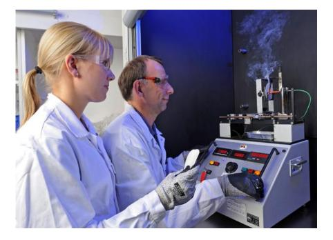
Services that LANXESS performs for its development partners include standard-compliant flame-retardant testing using methods such as glow-wire testing. These activities are part of the HiAnt service package that LANXESS offers customers to assist them throughout the entire development process for a component. Photo: LANXESS AG
