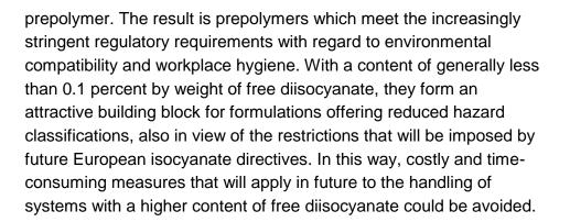
In addition, narrow molecular weight distribution and precisely adjustable prepolymer viscosity are, for example, important keys to optimized properties and improved processability. A better defined segregation of crystalline hard and amorphous soft segments in the coating compared to conventional prepolymers ensures exceptionally high film quality and durability.
