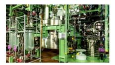
The paste bins in the Leverkusen production plant of Saltigo GmbH undocks the centrifuge and vertical mixer dryer as storage containers, thus reducing cycle times. Photo: Saltigo GmbH
