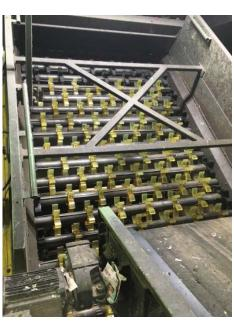
The PU star wheels based on Adiprene LF TDI are characterized by very high tear, abrasion and cut resistance and are resilient in humid and warm environments. Photo: LANXESS AG
