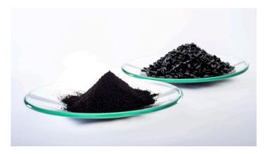
Specialty chemicals company LANXESS has developed a black pigment that reflects 20 percent more of the sun's near-infrared radiation (NIR) than conventional products. By means of coloring with Bayferrox 303 T (in foreground of picture), the service life of plastic components can therefore be extended, as they are less exposed to temperature fluctuations. Photo: LANXESS AG
