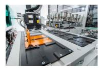
LANXESS is the world's only manufacturer capable of carrying out automated testing on the thermal stability of customer-specific formulations for iron-oxide pigments. Photo: LANXESS AG
