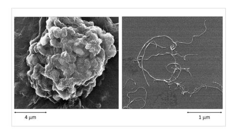
Electron microscope images of carbon nanotubes (CNTs) in agglomerated (left) and dispersed (right) states.
