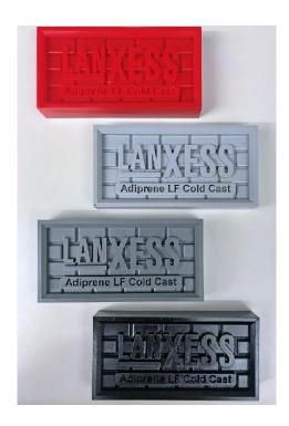
Samples of PU cast elastomers produced with Adiprene LF prepolymers and Vibracure curatives from LANXESS.
