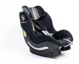
The child seat headrest has been developed as a technology demonstrator and is produced in a particle-foam composite injection molding process. The Tepex insert can reduce the weight of the headrest by up to 30 percent in comparison with the commercial component variant – and with comparably good crash performance, too. Photo: Professur Strukturleichtbau und Kunststoffverarbeitung an der Technischen Universität Chemnitz
