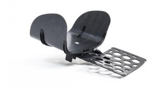
The Tepex insert is formed in a single process operation using an injection molding tool with turning plate and back-injected with a short-glass-fiber-reinforced polypropylene compound to integrate the support structure for the headrest and backrest, for example. Photo: Professur Strukturleichtbau und Kunststoffverarbeitung an der Technischen Universität Chemnitz
