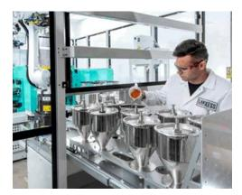
Consistent quality is a crucial requirement for plastics coloration. LANXESS ensures maximum product reliability by constantly monitoring the raw materials used and maintaining ongoing quality control using testing methods in accordance with global standards at its own in-house laboratories. Photo: LANXESS AG
