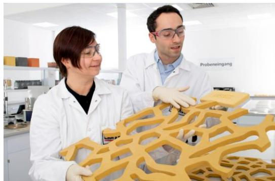
Color optimization in the application technology laboratory at LANXESS's site in Krefeld-Uerdingen. The lattice-like precast concrete element made from ultra-high-performance concrete (UHPC) is colored yellow using Bayferrox pigments. Tests prove that the strength of the meshed concrete structure is unaffected by the pigmentation. Photo: LANXESS AG
