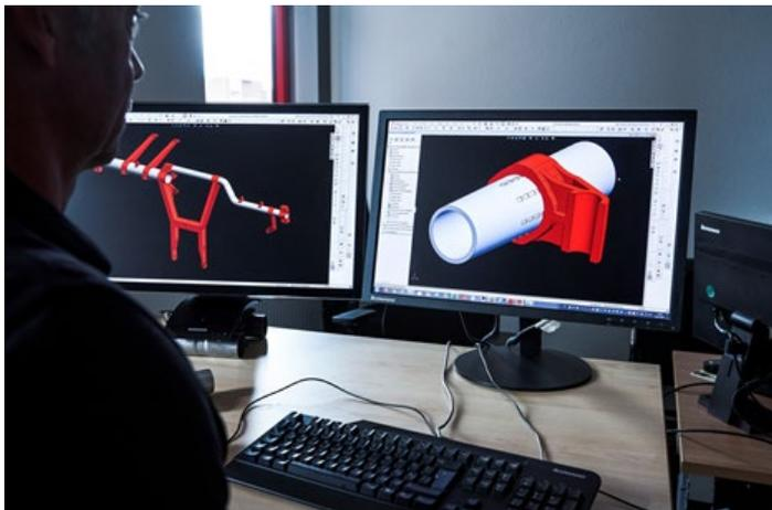
With its simulation tools, LANXESS is able to accurately predict the maximum stresses hollow-profile hybrids – such as automotive cross car beams (*left-hand screen*) – will withstand and at what point they will fail.
