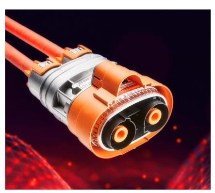
Connector made from Durethan BKV30FN04 for cable harnesses in electric models produced by a European-US automotive manufacturer. The halogen-free flame-retardant polyamide 6 can also be dyed in bright colors like orange (RAL 2003) and yellow and is characterized by its high strength and toughness.
