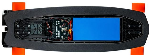
The trough-shaped deck houses all the electric and electronic functions, including the battery, except for the motors, which are mounted on the back of the skateboard.
