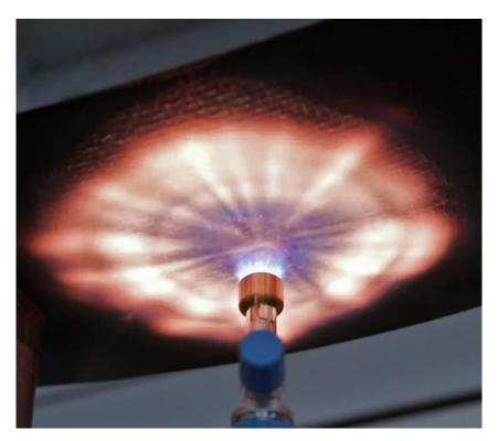
The reason for the good flame-retardant properties of Tepex is the high content of flame-resistant continuous fibers and the comparatively low proportion of flammable plastic.
